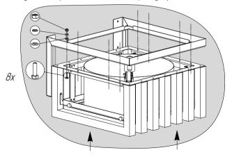
**3.2.** When fixing the device to the ceiling, mark the device's (1) attachment positions on the ceiling, considering the device's dimensions. Fix the device on the ceiling using fastening elements (not included).
