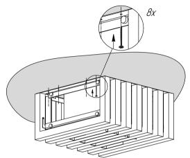
**4.** Install the decorative end plugs (3) in place. Attach the chain with the handle (2) via a latch hook to the device (1). Adjust the chain length, if required.
