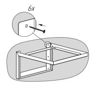
**3.1.2.** Install the bucket shower onto the bracket (7) and fix it using the fastening elements (included with the bracket) in eight places.
